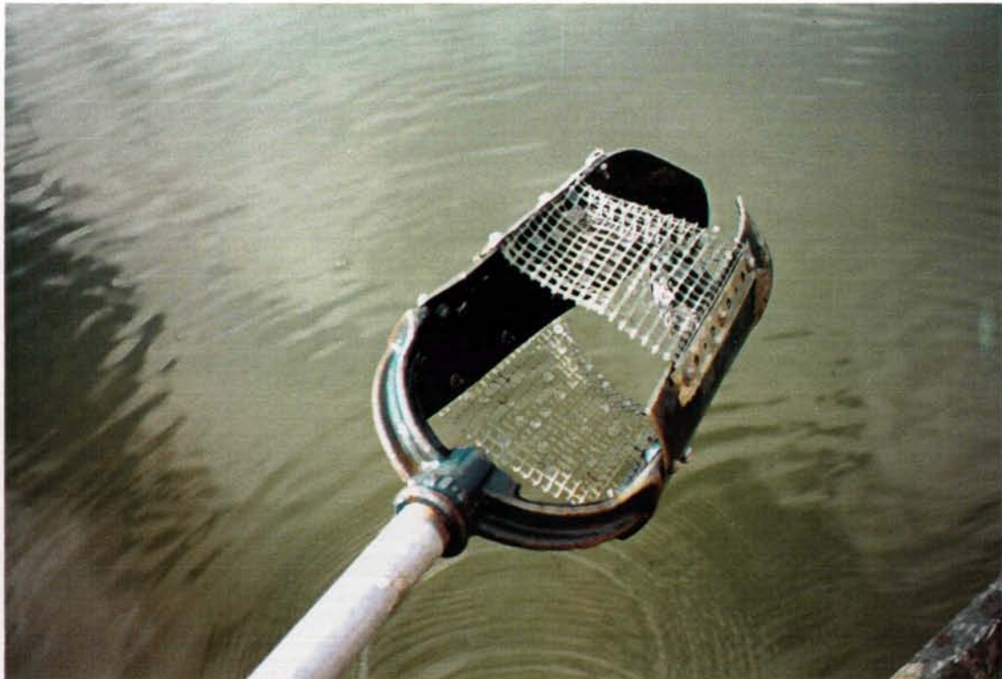
Figure 17. Modified soil auger (5-inch diameter) used to collect Powers Lake sediments.
