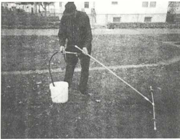
For small lakes or ponds, a distribution system for a buffered alum application can be constructed from PVC pipe. The buffered alum is mixed into a slurry in a pail and pumped through the manifold into the lake.
