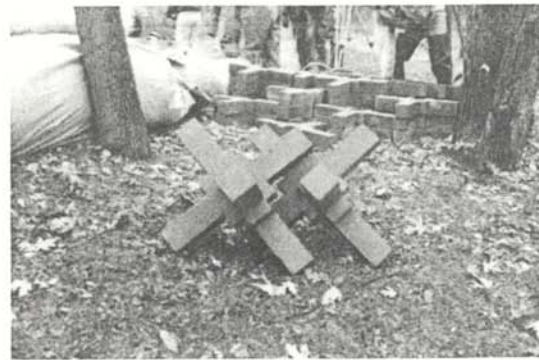
Another type of structural toe protection is the use of A-jacks. They are a good energy dissipater. As with rock riprap, they are permanent.
