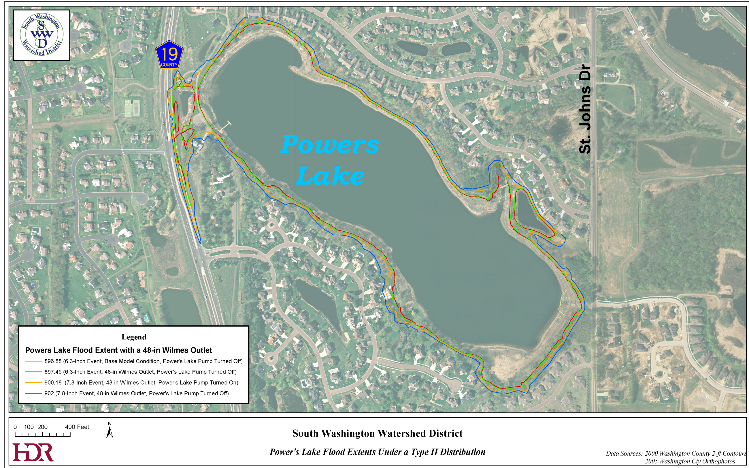
Figure 7 Flooding Extents and Duration at Powers Lake
