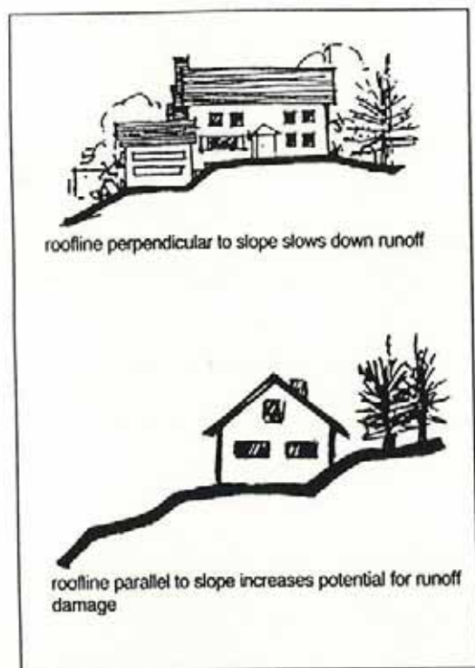
Figure 4: Build rooflines perpendicular to slopes
