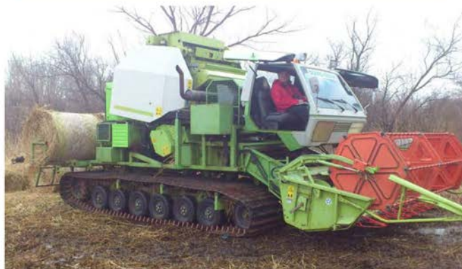
FIGURE 21. Bombardier trail groomer with front and rear hydraulics for powering implements.
