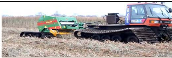
FIGURE 20. Modified Piston Bully harvesting reed ( Phragmites sp.) in Germany. Apparently, the unit converts hydraulics to run the PTO driven baler. Note the track-equipped baler and the supplemental radiator for additional cooling capacity of the hydraulic system.
