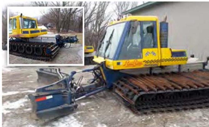
FIGURE 21. Bombardier trail groomer with front and rear hydraulics for powering implements.
