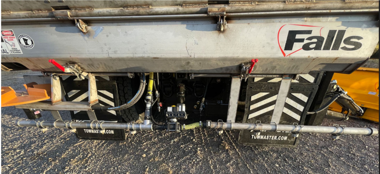
Above is a better look at the spray bar that is mounted to the rear of the plow truck. The spray bar is located underneath the salter of the truck. We currently do not have this on our plow trucks.
