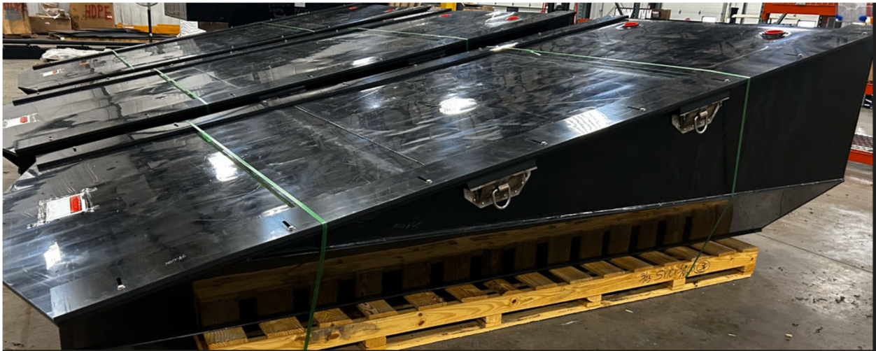
Above is a picture of the liquid tank while not before installation into the box of the truck.
